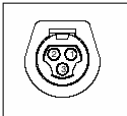
Figure 10. Hypertronics power receptacle, as viewed from the back panel of the NL100. Supply +24V DC on Pin 1. Pin 2 is the supply return and pin 3 is the case ground.
