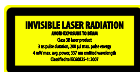
Figure 4. Laser information label, located on back panel.
